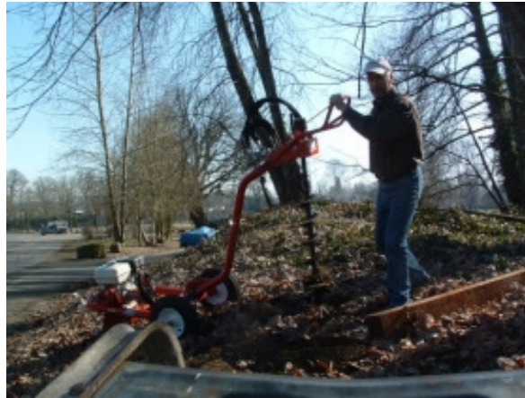
Russ Hall, above, director of Wilderness International Inc., deploys a post-hole digger at Meldrum Bar Park.
